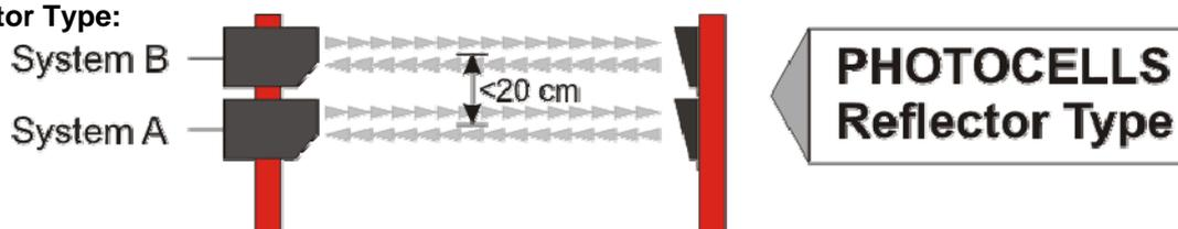
The reflector-type photocell has the transmitter and receiver electronics in the same case. A simple reflector on the opposite side of the finish line is used to reflect the photocell beam back to the main unit. For System A and B the reflectors should be on the same side.
